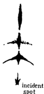
Fig. 1. The sketch of the electron diffraction pattern of the polished surface.
