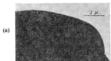
Phot. II. The shape and structural change of chrome-carbide powder during oxidation process.
